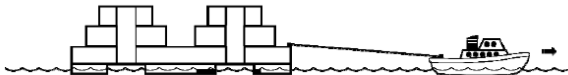
Figure 6: Towing of deck module
