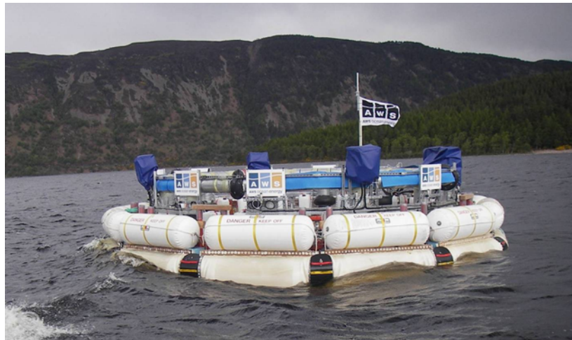
Figure 4.25 1:9 Scale model of the AWS-III under test on Loch Ness, June 2010 [50]
