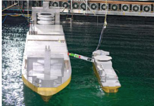
Figure 186: Channel testing of the Accommodation Vessel model Dan Swift . Source: Offshore Lauritzen A / S
