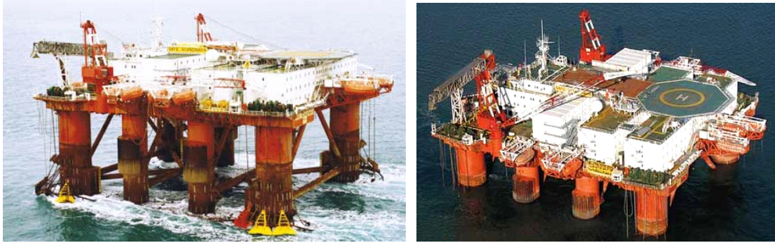
Figure 96: Safe Scandinavia floater. Load shedding for transport and operating weighted in draft.
