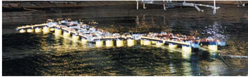
Figure 124: Tests to evaluate hydroelastic connectors (59)
